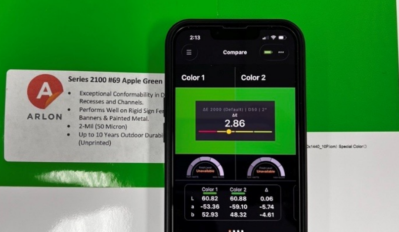
COLOR 1 (LEFT): Arlon Series 2100 #69 Apple Green color vinyl target. COLOR 2 (RIGHT): Omni Cast Wrap digital print output.
