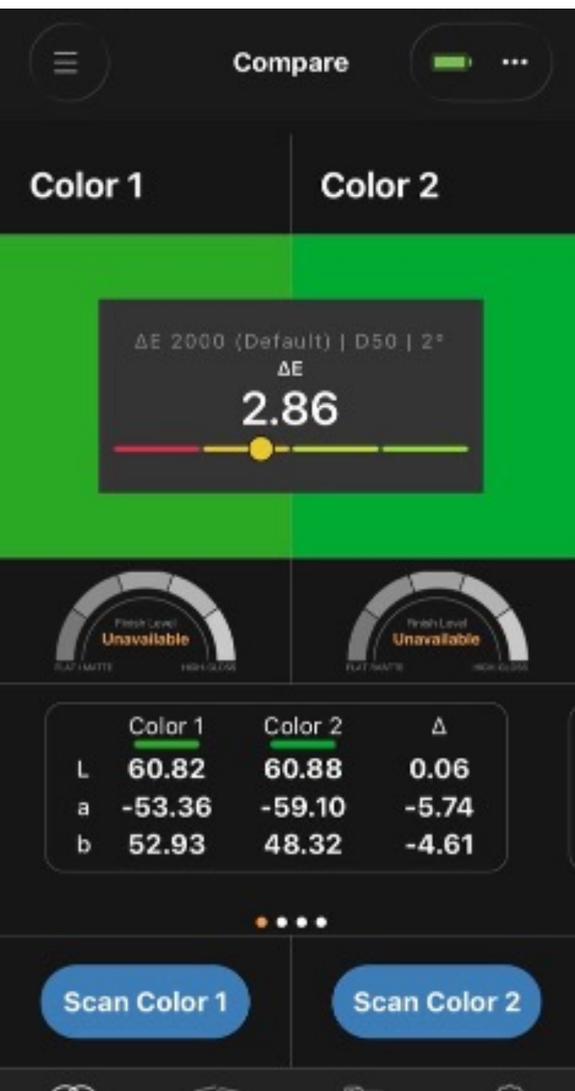
COLOR 1 (LEFT): Arlon Series 2100 #69 Apple Green color vinyl target. COLOR 2 (RIGHT): Omni Cast Wrap digital print output.
